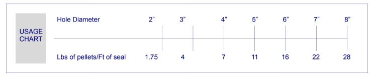
NOTE: These are dry weights and volumes. In use, the swelling of the pellets will increase the length of the seal (depending on hole condition).
